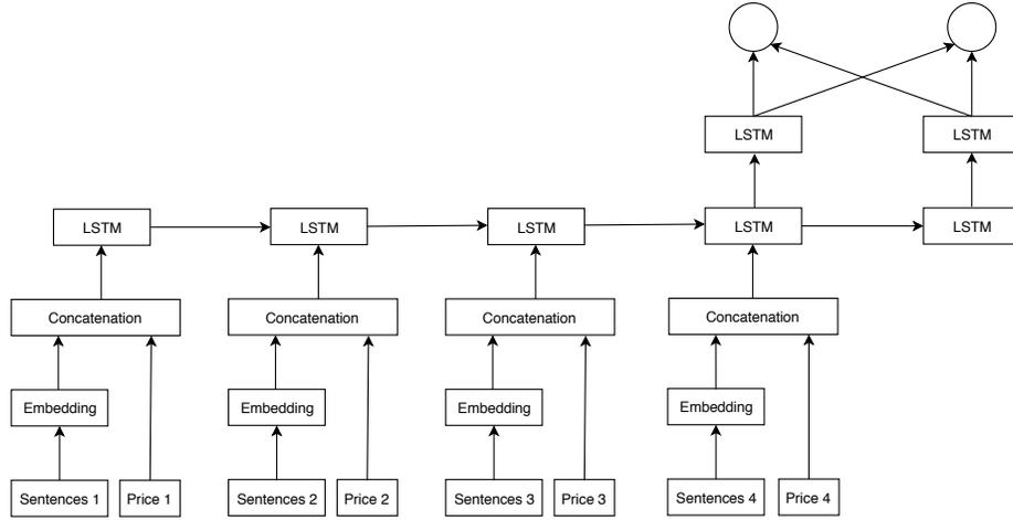
Fig. 3: A demonstration of the stacked LSTM structure. In this example, it uses data of four days to predict the gas price of the next two days
