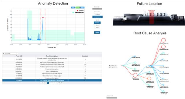
Figure 4. Event Data visualisation. The time plot in the upper left shows the event frequency within a day, and the statistical normal model in the background. The company-internal failure data catalogue has been linked into the lower left and on the right side are the results of the correlation analysis [14] (Screenshot provided by Marco Huber, USU Software AG, Germany)
